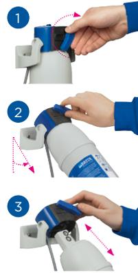
To exchange the filter cartridge, rotate the locking handle to divert the water and release the cartridge. Press the flush valve and depressurise the filter. Remove the filter cartridge from the filter head.
